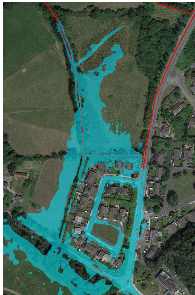
Figure 9.7: Flood mapping based on existing topography (stream flow at 0.1% AEPCC, river flow at 10m 3 /s)
